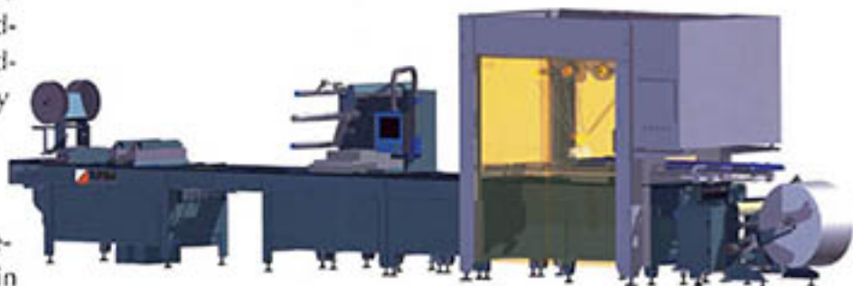
I-Load island automatic loading system (Ilpra).
